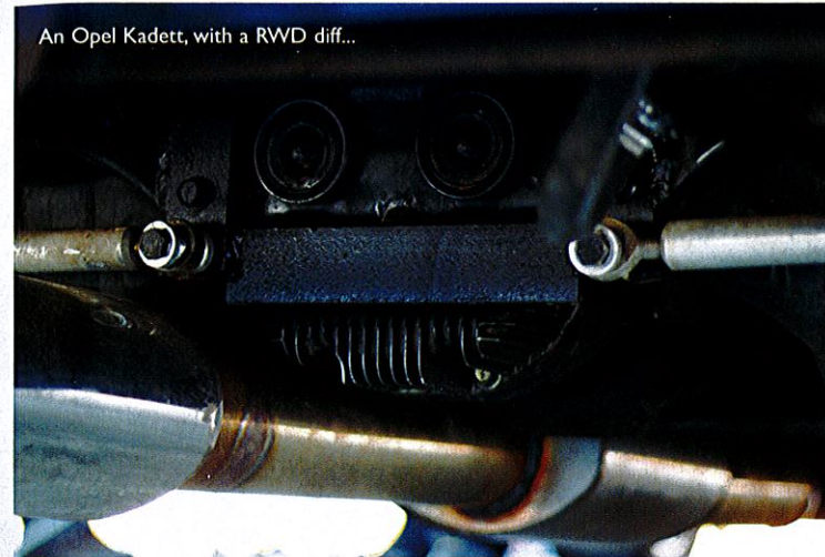
Rose jointed suspension for added strength.
